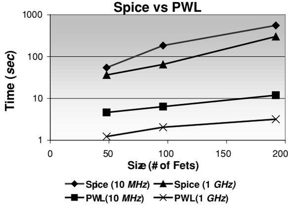
Fig. 4: Spice vs. PWL Models in a System of Multiple FETs.
