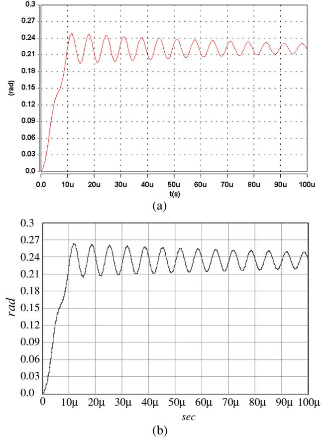
Fig. 6: Transient Response of a Beam: (a) NODAS (b) Chatoyant.
