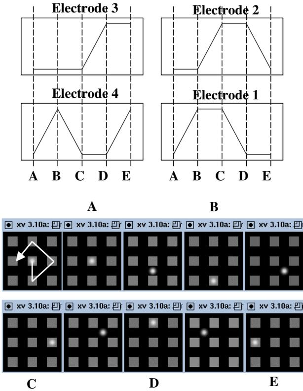
Fig. 16: Scanning Waveforms and Scanned Diamond Pattern.
