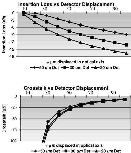
Fig. 12: Insertion and Crosstalk vs. Mechanical Tolerancing.
