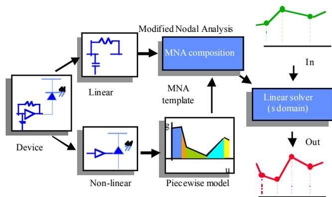
Fig. 1: Piecewise Modeling for Electrical/Optoelectrical Devices.
