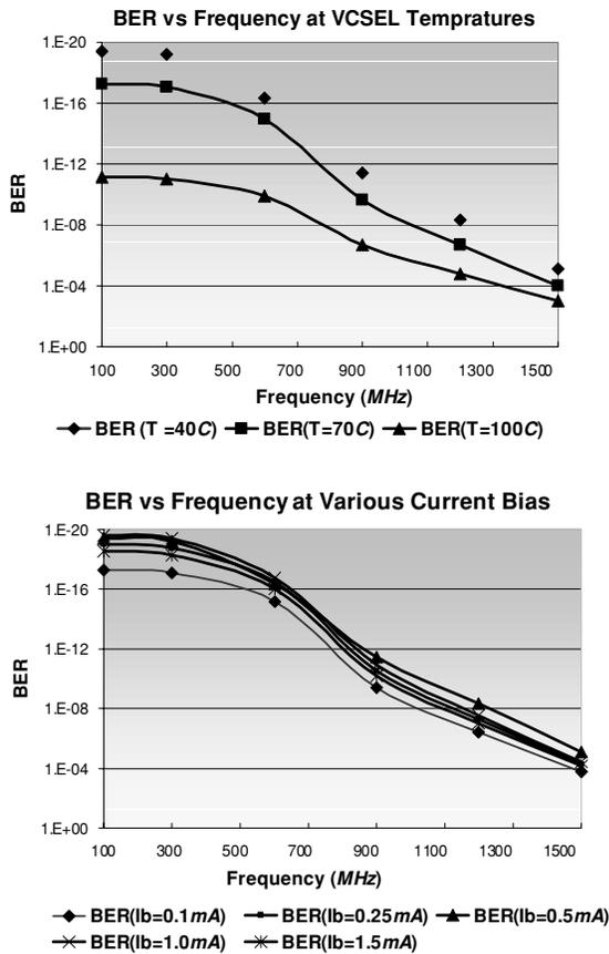
Fig. 11: BER vs. Frequency at Different VCSEL Temperatures and Current Biases.
