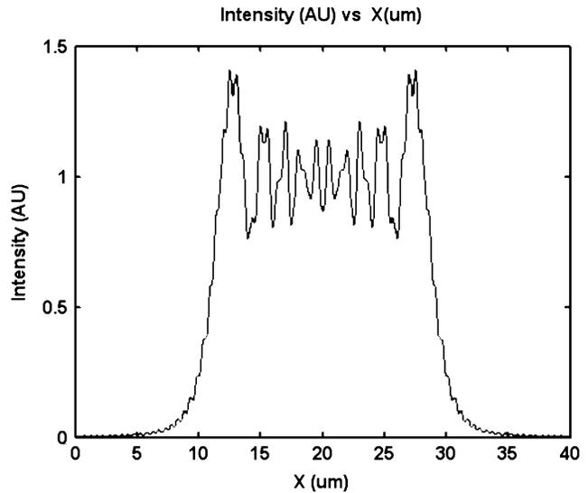
Fig. 7. Power distribution simulation at the fiber interface.
