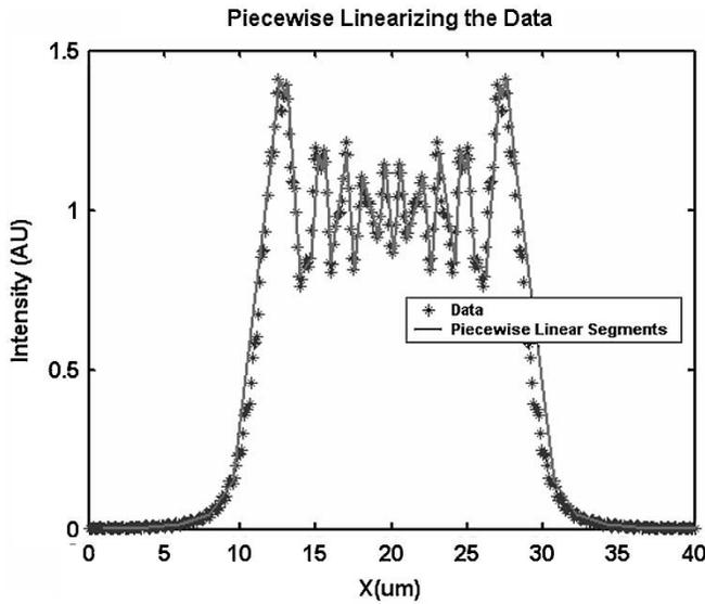
Fig. 5. PWL segments of the optical power distribution.
