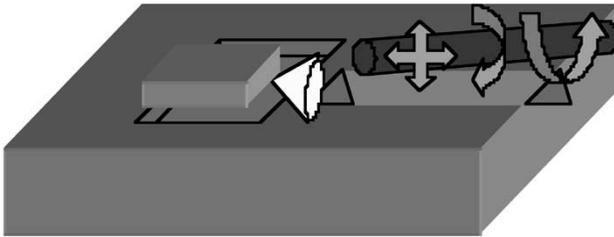
Fig. 6. Edge-emitting laser coupled to a fiber.
