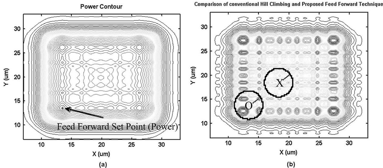
Fig. 8. (a) Contour diagram of the power coupled into a 4- $\mu$  m fiber determines the feed-forward set point. (b) Intensity contour of wavefront with superimposed final fiber positions using the current state-of-the-art technique (“X”) and our knowledge-based control algorithm (“O”). Using our proposed technique, we show an improved system performance of approximately 18%.
