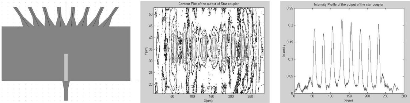
Fig. 10. Star coupler and optical intensity contours shown in 3-D and 2-D.
