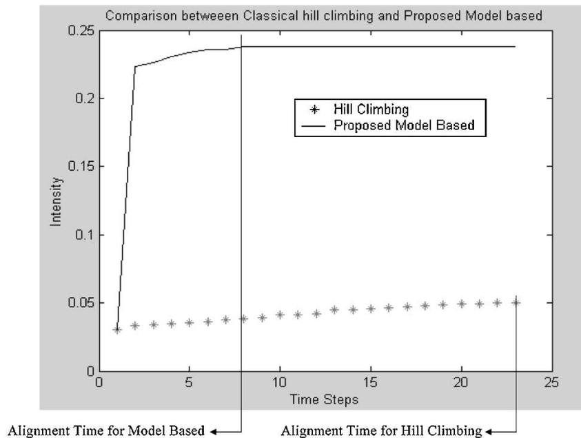
Fig. 12. Iterative time step comparison of our knowledge-based control method versus existing alignment control.
