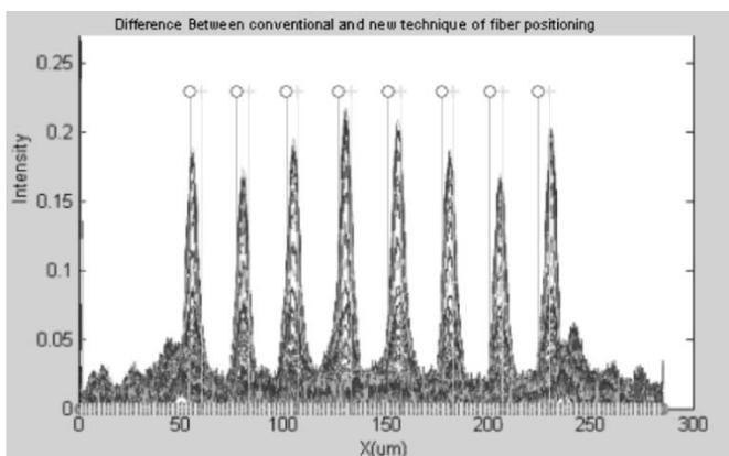
Fig. 13. Fiber array alignment of the hill-climbing algorithm (dark lines and “o” shape) and our knowledge-based control loop (light lines and + shape).
