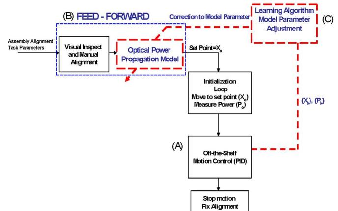
Fig. 1. Model-based control algorithm for automation of photonic systems.
