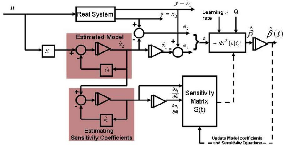
Fig. 2. Simulation of the learning loop technique [2].
