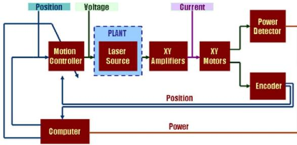
Fig. 8. Hardware setup.
