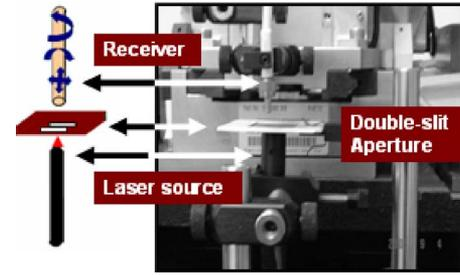
Fig. 9. Laser source being coupled to a fiber through a double slit.
