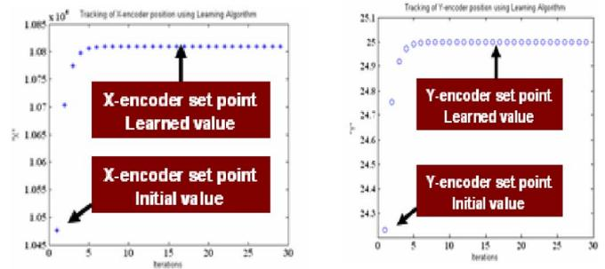
Fig. 12.  $X$  and  $Y$  encoder set points.
