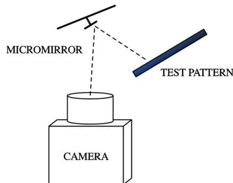
Fig. 2. (Color online) Relationship between the camera, the array, and the test pattern.
