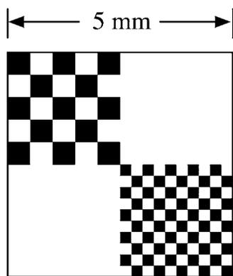
Fig. 1. Fundamental unit of our test pattern. A checkerboard pattern was chosen to allow for calibration. The two different size checkers illustrated that the resolution of the device was between 0.5 and 0.025 mm.
