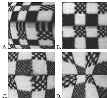
Fig. 3. Image,  $160 \times 160$ , created by scanning the test pattern with a single mirror and uniformly spaced voltages. B, Image,  $129 \times 129$ , obtained by using a nonlinear voltage table. C, Fisheye distortion can be introduced by transforming the voltage table in a radial manner. D, Pincushion distortion introduced by transforming the voltage table appropriately.
