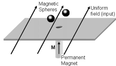
Fig. 1. Magnetic assembly and manipulation system illustration.
