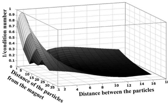
Fig. 3. Controllability map of two-particle system when particles remain above permanent magnet at height of 1 radius. External field is applied in  $x$  direction. Distances are measured in 0.2 particle radii.
