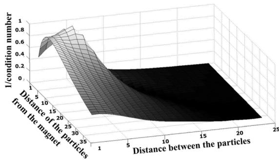
Fig. 2. Controllability map of two-particle system when particles remain above permanent magnet at height of one radius. External field is applied in  $y$  direction. Distances are measured in 0.2 particle radii.
