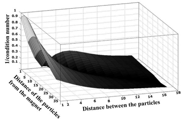
Fig. 4. Controllability map of two-particle system when particles remain above permanent magnet at height of four radii. External field is applied in  $y$  direction. Distances are measured in 0.2 particle radii.
